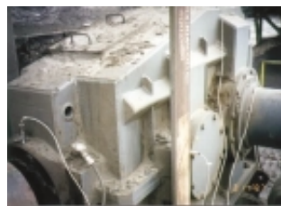
Figure 1: Typical sensor positions during vibration analyses on the bevel drive
