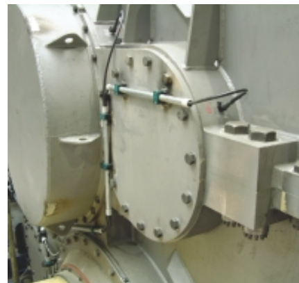
Vibration Accelerometers on rolling bearings
