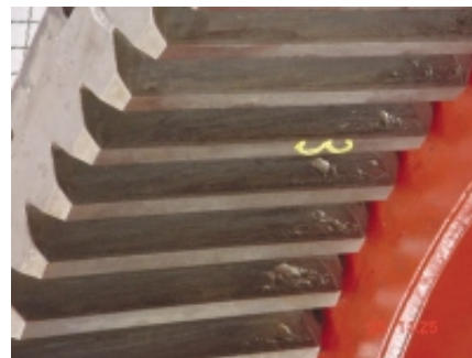
Figure 4: Unbalanced tooth damage on the internal gear
