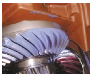
Fig. 3 Ideal result of the contact pattern check
