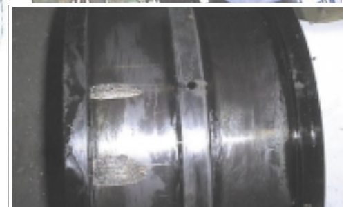
Fig. 4: Inner raceway with diagnosed pittings
